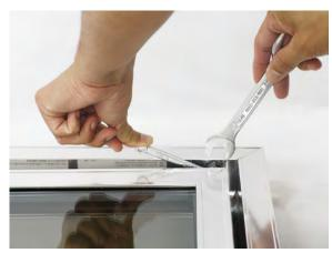
Figure 2. Adjust tension using wrenches
